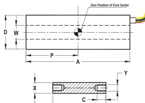
**NOTE**: Output will be positive when core moves from zero toward lead wires end of LVDT
